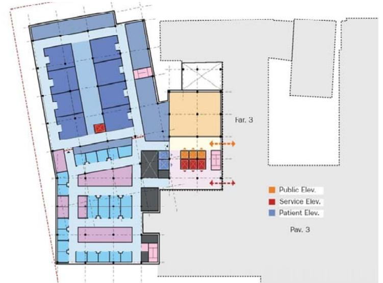
Floor Plan Level. 3: Operating / Procedure Platform
