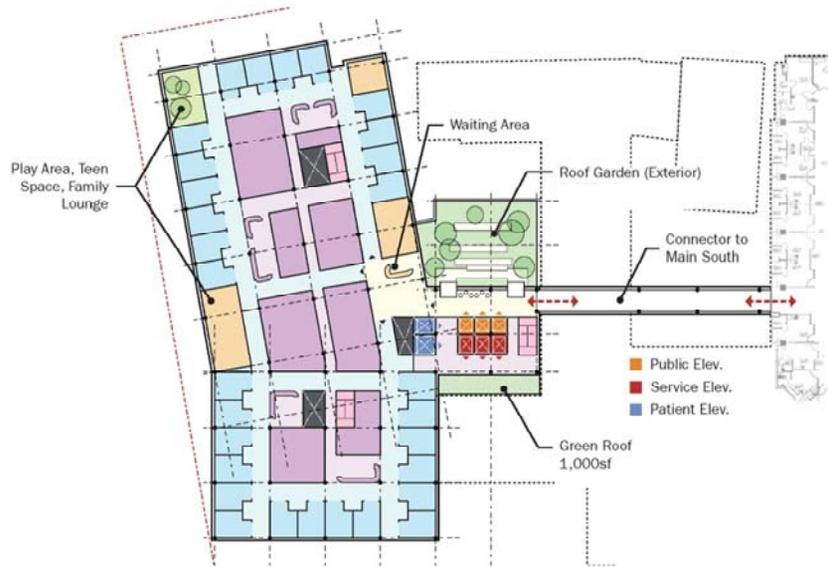
Floor Plan Level. 9 (10 & 11 Sim.): Typical 30 Bed Unit
