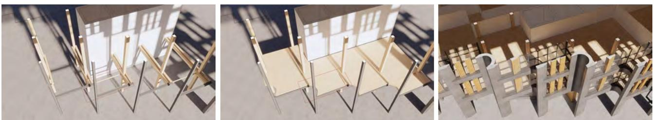
Cantilevering double glulam beams combined with steel beams and columns allowed for a separate CLT panel for the concaved balconies.
